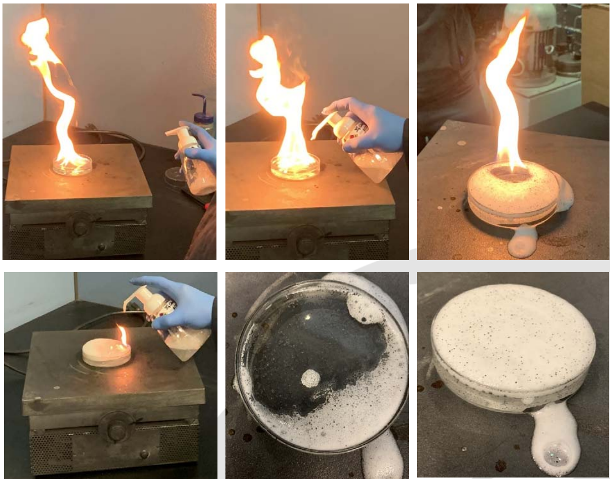
Figure 2: Before, During, and After Extinguishing Kerosene Fire Using STAX®-Based Firefighting Foam (Black Specks are Expanded Graphite Worms)
