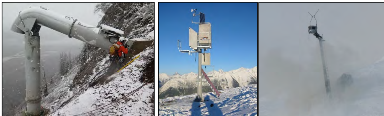
Figure 4-1: Three separate RACS systems for triggering avalanches – Gazex (left), Avalanche Guard (center), and Wyssen Tower (right)
