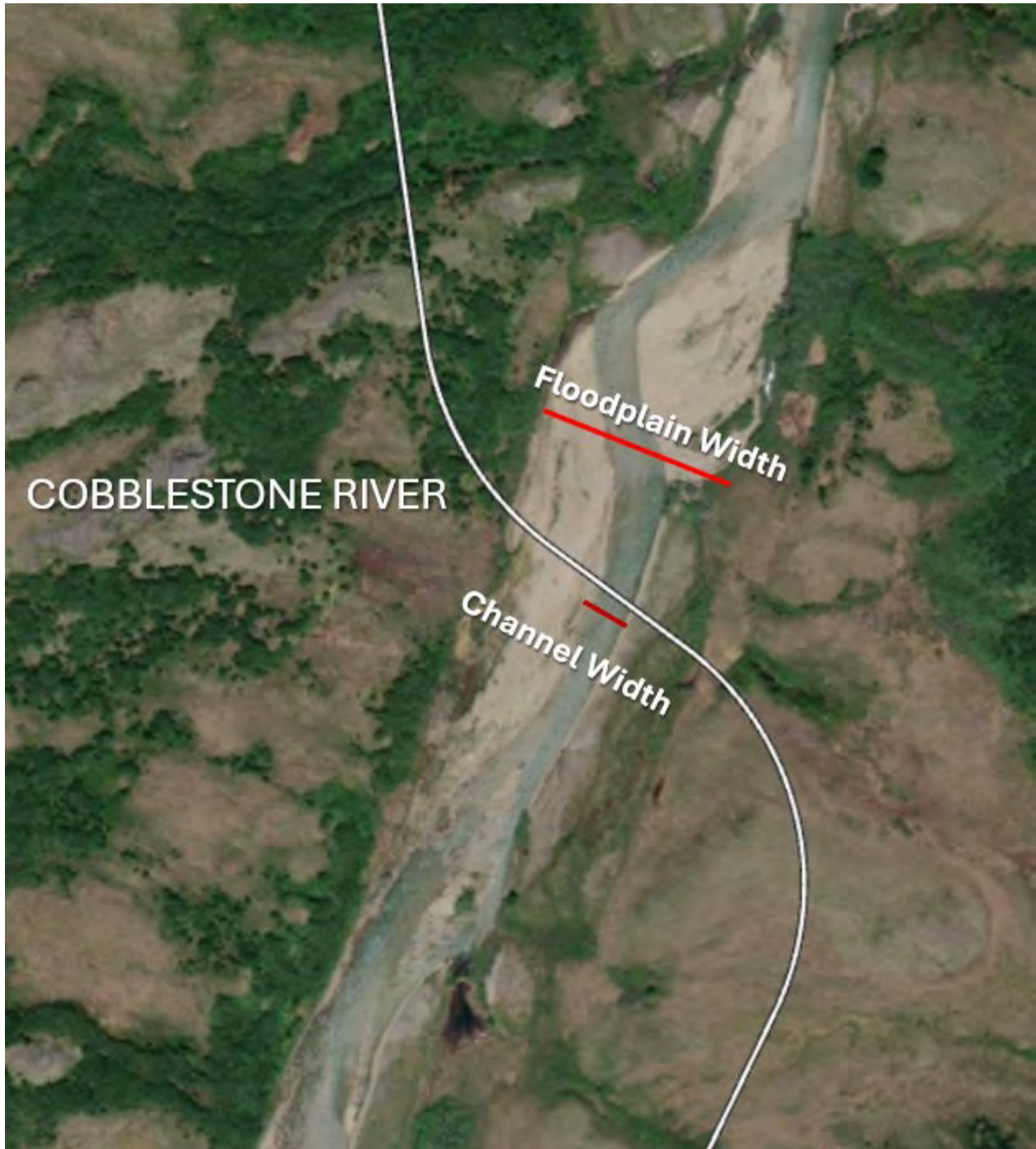
Figure 3-10. Cobblestone River alluvial channel with active gravel bars
